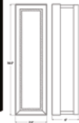
HF9404-BLK Black 16.5"H x 7.5"W x 4" Ext OAH 16.5" 17 Watt / 12V 3000K / 90 CRI 550 Lumens
